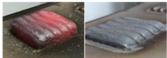
图11 堆焊后零件尺寸形貌 Fig.11 Dimension of welded parts
